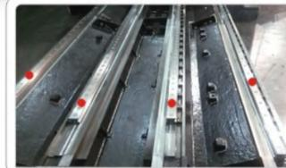
Both X and Y axis equipped with high quality linear guide way, the machine bed use four linear guide ways to provide great support for the worktable, it also increases worktable's loading ability and lower the vibration while cutting.
