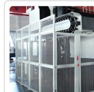
ATC is designed with safety enclosure guard and safety switch in order to protect the operator (For example, if the door is opened during running, the machine will stop automatically)
