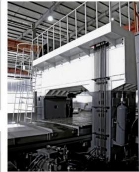
On the back, a ladder and other safety devices simplify maintenance of the machine. Seamless steel pipes provide clean, efficient and fast oil circulation.
