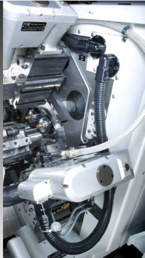
Motorised cross slide fine adjustment for the correction of dimensional errors and for tool wear offsets
