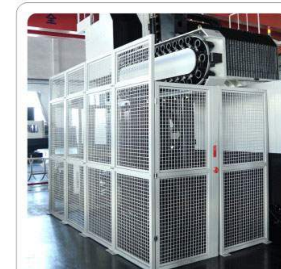
ATC is designed with safety enclosure guard and safety switch in order to protect the operator(For example, if the door is opened during running, the machine will stop automatically)
