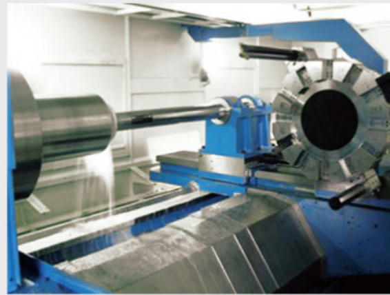
Deep Hole Boring
