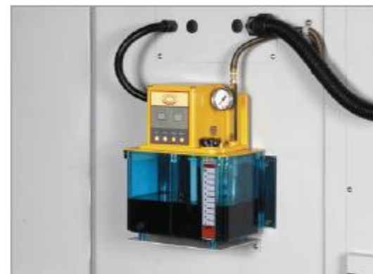
供油系統 Automatic lubrication system
