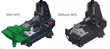
Considering the requirements of cycle time and loading/unloading time, an APC (automatic pallet changer) system is available as an option.
