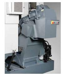
Coolant tank capacity: 700 L(80% full)
