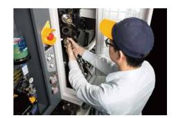
A big size tool magazine door design facilitates tool checking and replace-
