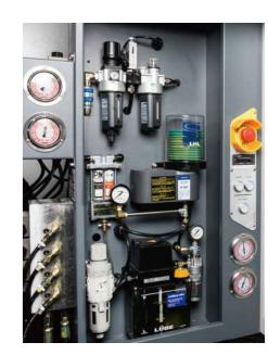
Through centralized management of air FRL unit and lubrication pump, daily maintenance becomes easier.
