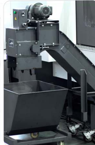
2 sets of coil chip conveyor intergrated with machine bed combine with set chip conveyor
