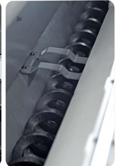
2 sets of coil chip conveyor intergrated with machine bed combine with set chip conveyor
